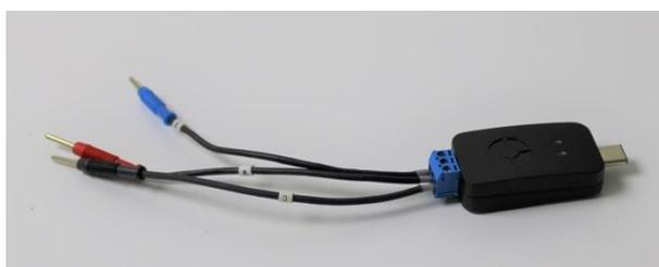
Figure 3.2 Sensit Smart and screw terminal assembled
